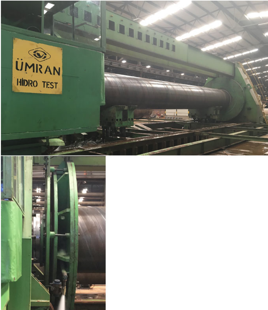
Fig. 12.4 Hydrostatic test setup
